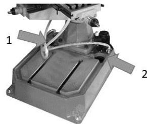
The coolant can be filled at the base at the two marked points (1,2) - see picture on the left.
