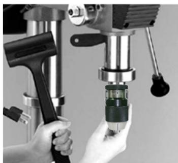
4. Mounting/removing drills / morse taper:
