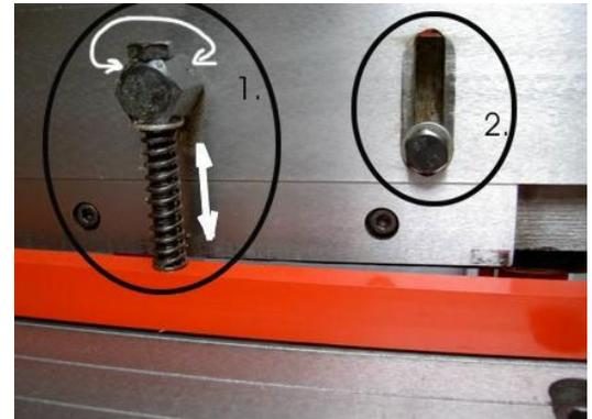
To set the cutting table loosen the screw and adjust the table to a position so that the blade has a free run. After the setting retighten the screw
