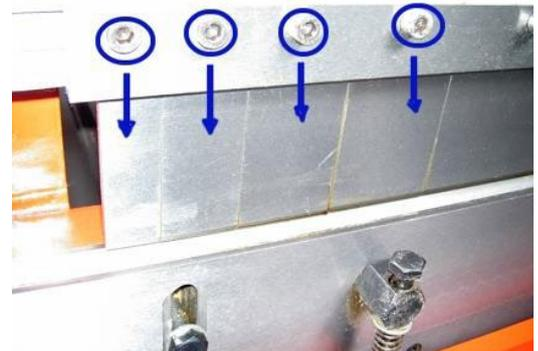
For rolling function the rear and upper roller can be adjusted. To adjust the distance and thus the roll diameter use the set screw at the rear side of the machine. If this role is not adjusted in parallel, for example, conical shell are produced.
