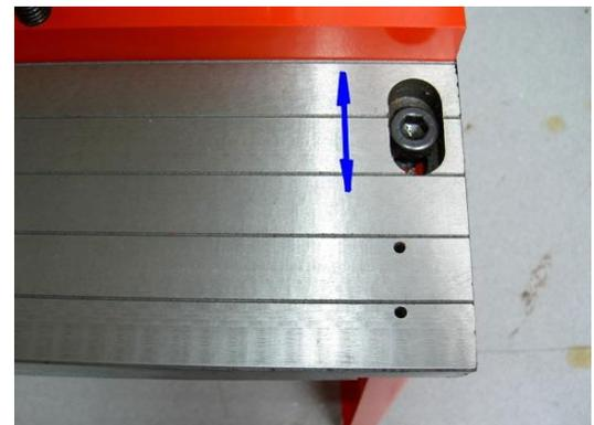
For bending the different segments can be removed or replaced, depending on workpiece size, so that a defined bending edge can be generated. For this purpose, loosen the screw of the corresponding segment to move or remove this. After new setting retighten the screw.
