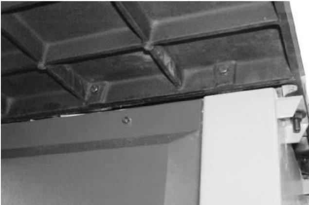
Mount the table bracket using **4 M8x20** screws / washers on the sliding table.
