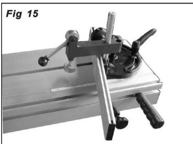
Now adjust by means of **4 M12** hexagon screws **C** the table bracket so that it is in line with the format table. Check this place by means of a planar object over both control and with a spirit level. If you are satisfied with the setting, don **C**.
