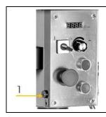
• By pressing the button for ccw-direction (1), located laterally on the control panel, the rotation direction of the drill bit changes into counterclockwise rotation direction.
